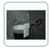
While operating the GSM finder the operator fixes the antenna on the breast or on waist in front. Turning to the right or to the left will achieve maximum signal
