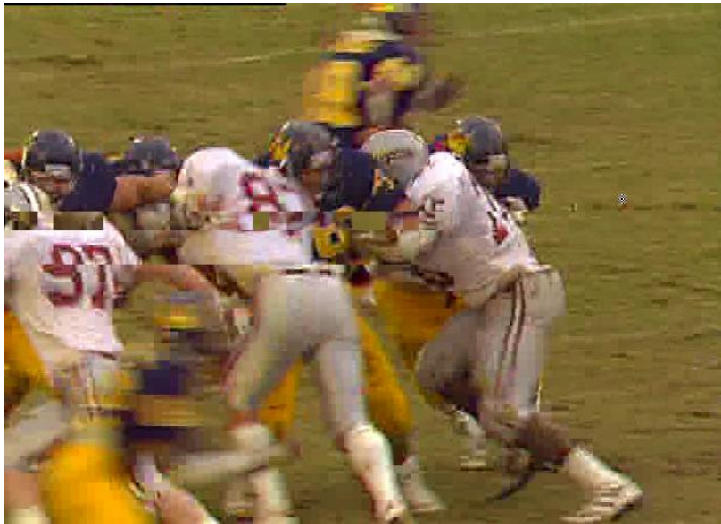
Single B-frame IP packet loss (at 3.1 seconds, 1 frame affected)
