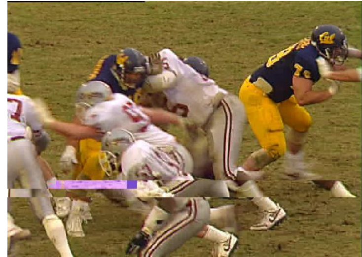
Single I-frame IP packet loss (at 2.4s, 14 frames affected)
